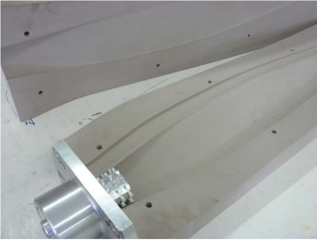
Figure 5. Finished propeller blade molds
