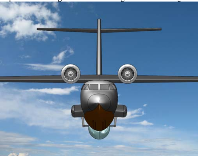
Figure 2: Example of CAD model with retractable floats
