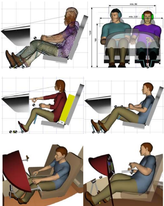
Figure 4. Reference dimension for small aircraft with adjustable seats and/or adjustable pedals
