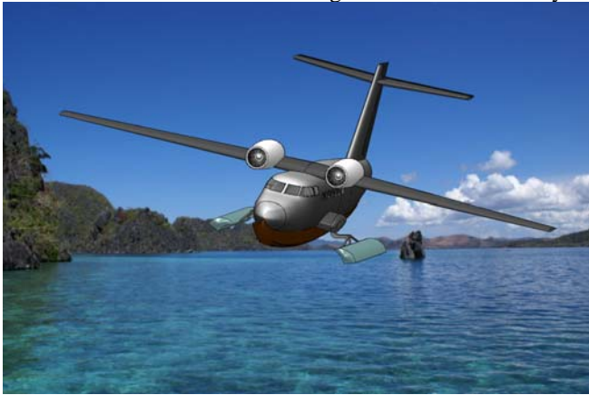
Figure 6: Seaplane CAD Model showing Trimaran Hull
