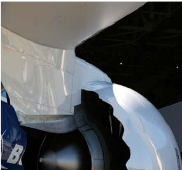
Figure 4. end-pass channel for suppressing noise blowers Trent 1000
